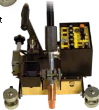
KBUG-1067 Magwheel Kit for welding curved or irregular shapes
