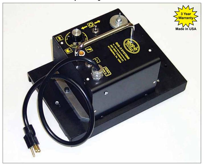
The **BUG-O DC IV** is a dual speed range, positive rack & pinion drive, ready for mounting welding or cutting attachments and accessories. It consists of a DC IV Drive unit mounted on a 12" (305 mm) Carriage. This unit runs on standard Aluminum Rigid Rail & Aluminum Flex Rail.
